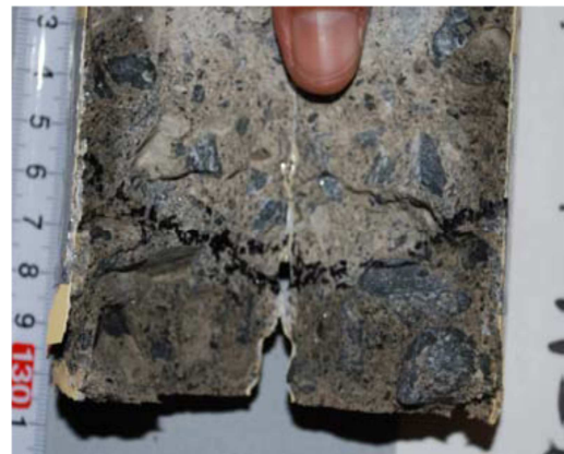
Figure 9. Fraction surface of the test specimen.
